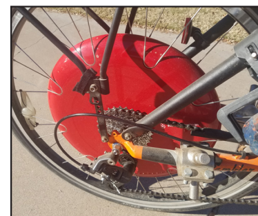
Closeup of Installed Copenhagen Wheel
